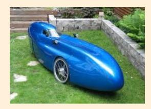
small roof and even rain and sun stay off of the rider. Combine this with the stability of three wheels and it allows riding in light snow while staying dry and warm.
